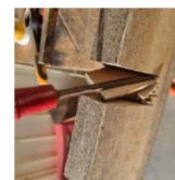
Back with the first backrest component. After running the saw through the rebate marks a few times I then go in with the chisel to remove the wood. Running the saw through makes the wood weaker and easier to run the chisel through.
