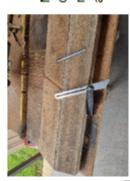
Next, I am once again using the chisel to create another rebate in a different position on the legs this time. This 30 degree chiselled rebate allows the main seat component to slide in being sturdy and/or reliable.
