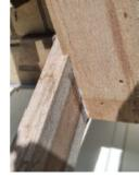
This is a key factor or the build, this image on the left is indicating and showing the rebated joint, as the seat component is slightly conjoint and merging with the right front leg with a "truss head" screw and more PVA wood glue keeping it in place.
